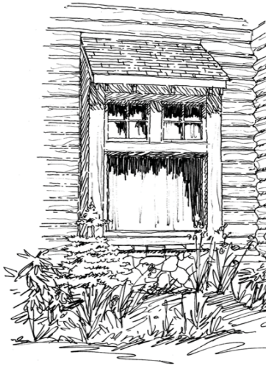
Shed-roofed Window bay
