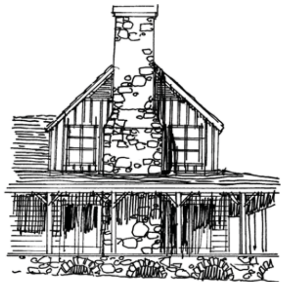
Vertical & horizontal siding accentuate the massing
